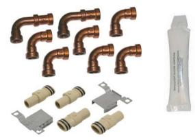
The threshold kit is used to join two sections of ThermaSkirt® when crossing a doorway, arch or fireplace, etc. Ensure that feed and return pipes are installed correctly (obtain a template from www.discreteheat.co.uk/technical.data.html) making sure you allow for carpets or tiles if not Finished Floor Level (FFL).
